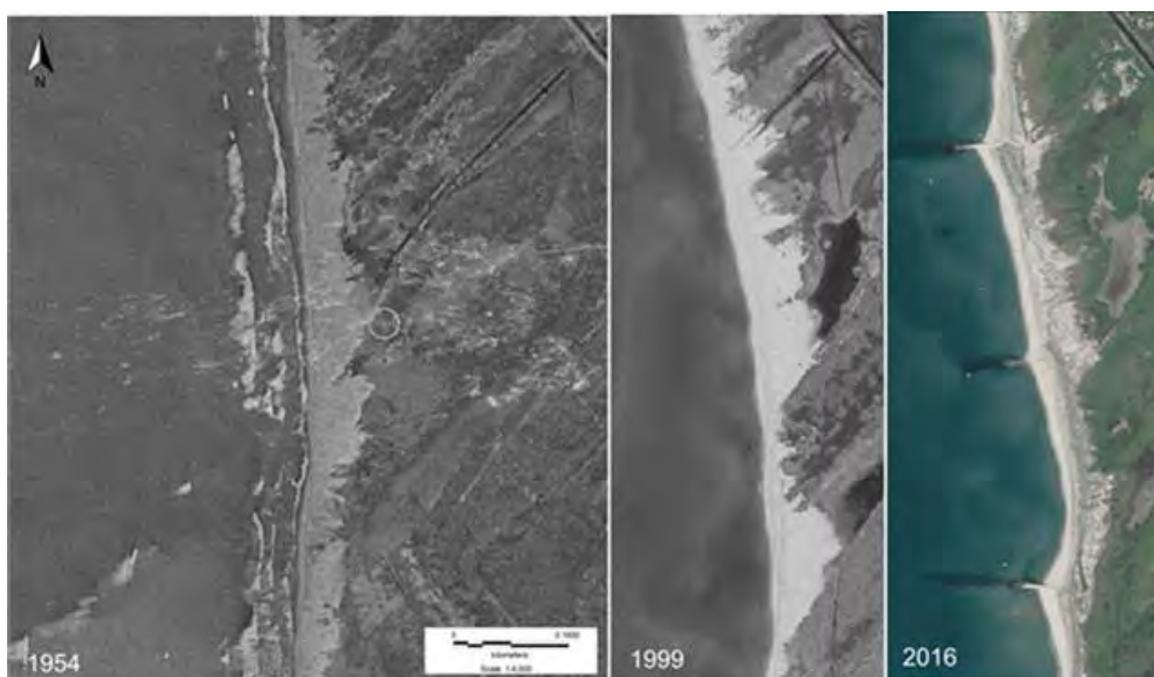
**Figure 4.** Effects of orthogonal breakwaters on erosion restraint. Aerial photos are from <http://www.regione.toscana.it/-/geoscopio> and licensed under Creative Commons Attribution CC-BY3.0 IT.
