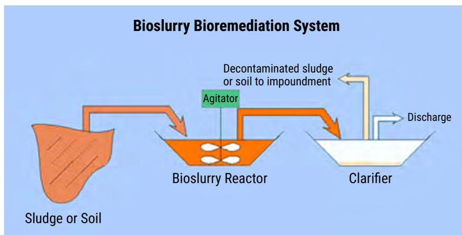
Schematic of a bioslurry bioremediation system. Source: Adapted from the U.S. EPA (8).
