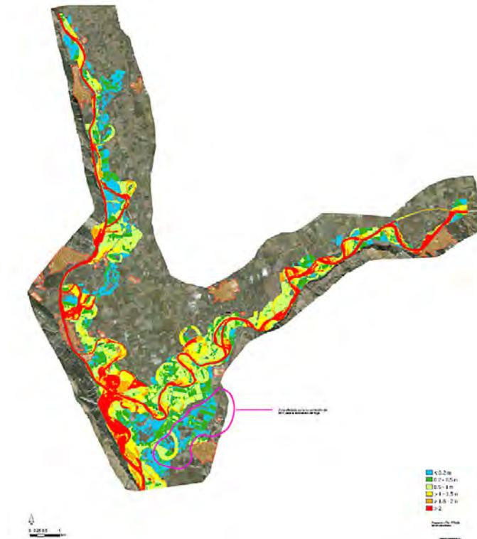
**Figure 4.** Example of the hydraulic, geomorphologic and ecologic modeling conducted for the design of restoration alternatives in the Arga-Aragón river system (CEDEX, 2010); in the provided image, for a return period of 10 years. Many of the restoration measures selected were aimed to increasing the water & sediments retention capacity of floodplains, and to allow a better protection of consolidated urban areas and certain critical sections.
