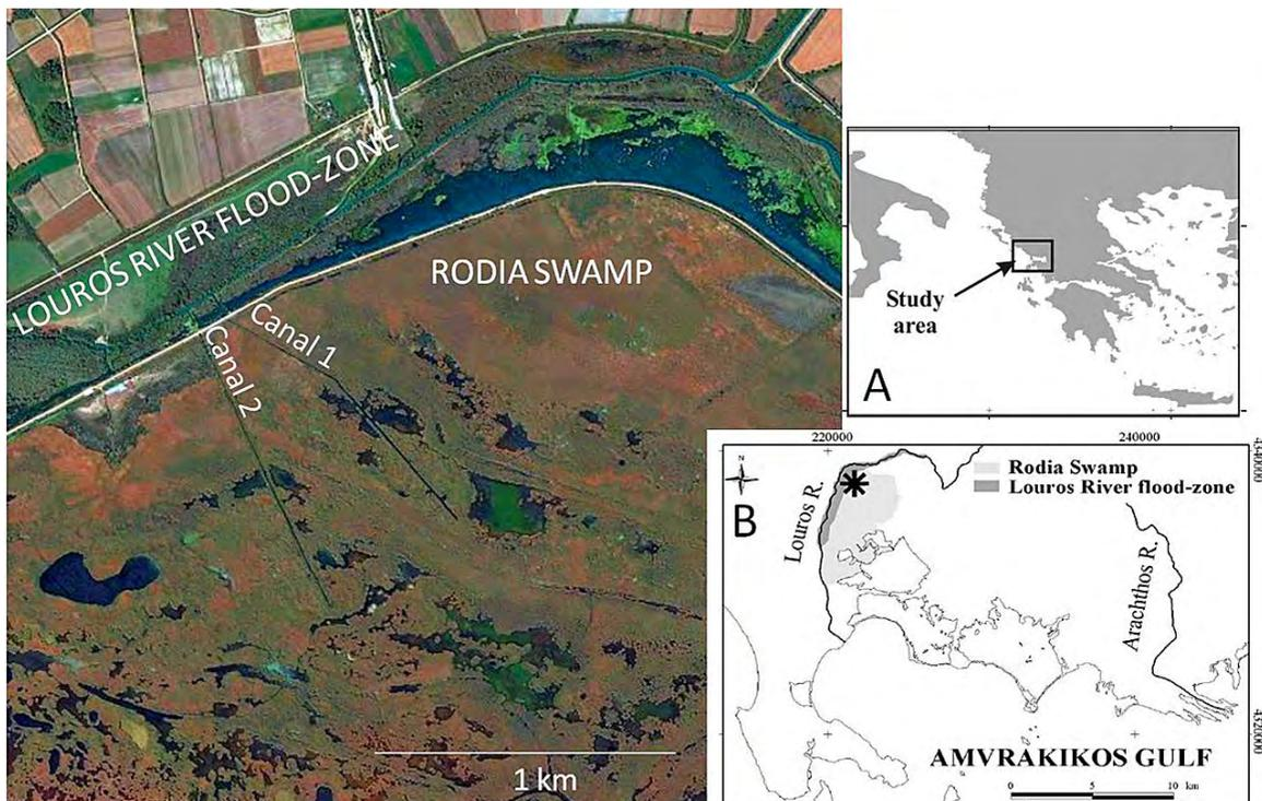
**Figure 1.** Google Earth image (2005) of the project site, showing the two new canals emanating from the embankment. Inset maps: A. The Amvrakikos Gulf along the west coast of the Balkans; B. Detail of the Northwestern Amvrakikos Gulf with the Rodia Swamp and the Louros River flood-zone (the asterisk shows the site of the restoration intervention where the sluice-canal system was constructed).
