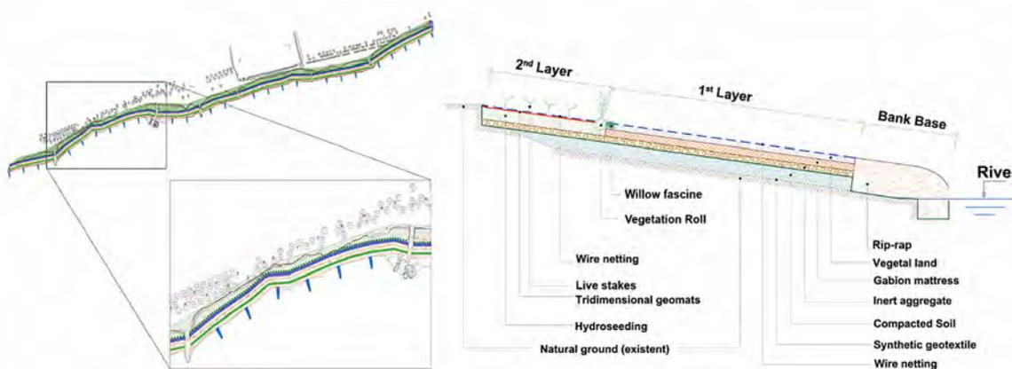
**Figure 3.** General view of the intervention area at Cardielos site (left, view from above, which highlights the row of deflectors and groynes and the bands dividing each intervention; right, transversal section exhibiting in detail the techniques used in each band.
